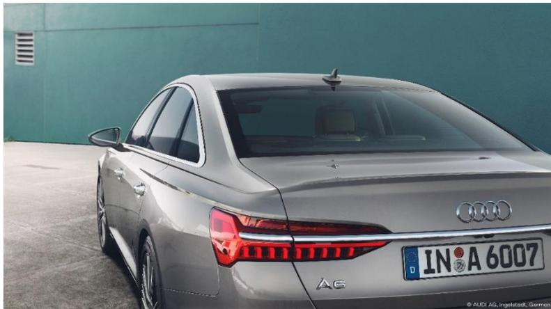
odelo was awarded the 2019 GKV/TecPart Award for the taillight in the Audi A6. The automotive supplier bonded the component made from PLEXIGLAS® molding compound using an innovative laser welding process.
